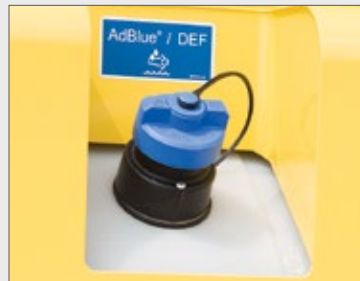
Diesel Exhaust Fluid (DEF) tank
