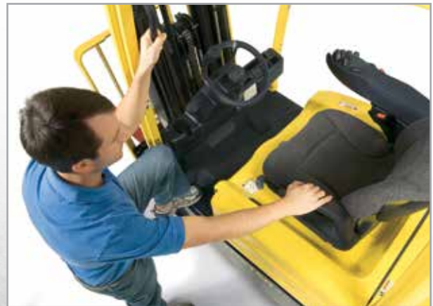
Three-point entry into operator compartment
