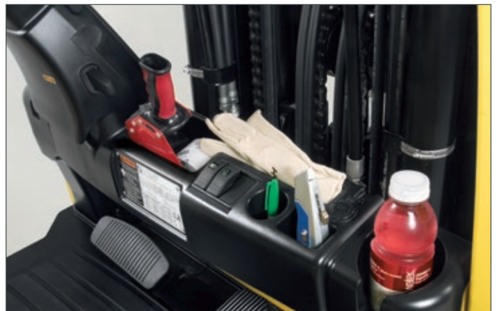
Operator convenience station
