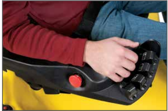
Electro-Hydraulic Controls with TouchPoint Mini-Levers
