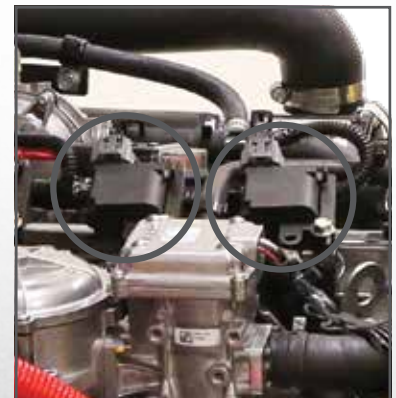
Coil over plug ignition design
