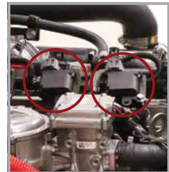
Coil over plug ignition design
