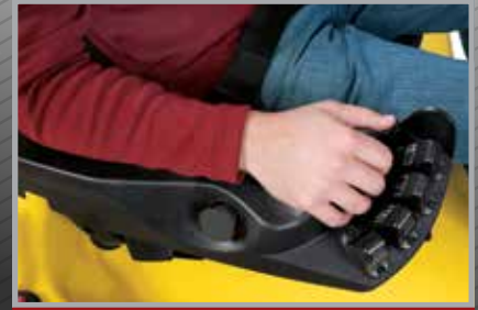
Electro-Hydraulic Controls with Touchpoint Mini-Levers
