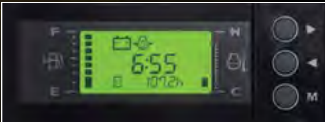
Integrated dash display shows error codes and warning indicators, reducing downtime to perform truck diagnosis.
