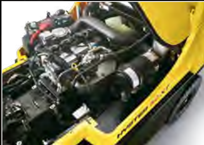
Rear-opening, one-piece hood and easy-to-remove, one-piece floor plate which requires no tools.
